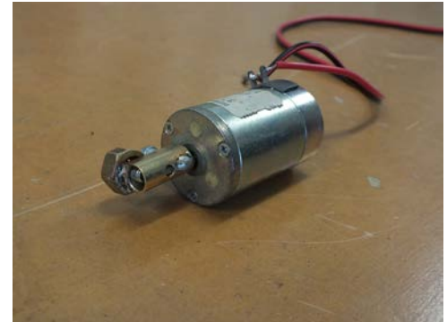
Figure 9. Fisher, H. (2016). Custom made vibration motor
